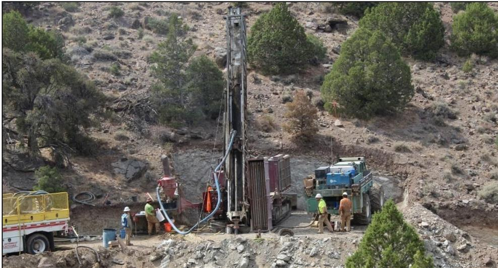
**Figure 1.** Reverse Circulation drill rig at the southern end of the Hercules target.
